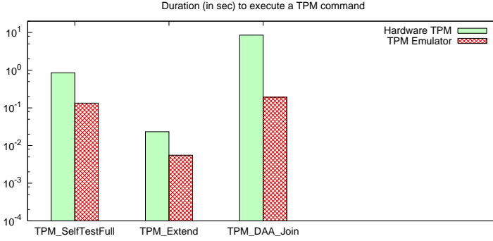
Fig. 4. Performance comparison of the emulator with a hardware TPM v1.2
